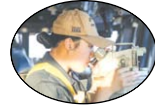
Ensign Nicole Choi looks through a telescopic alidade on the bridge of USS Dewey. U.S. Navy photo by MC1 Greg Johnson
