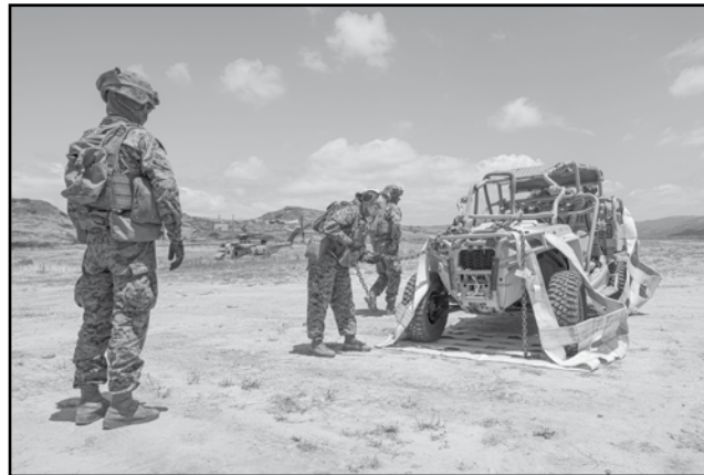
Marines assigned to Combat Logistics Battalion 15, rig a Polaris MRZR, an ultra-light turbo diesel combat vehicle, with a wheel net for lift operations with a helicopter support team on Camp Pendleton May 9. CLB-15 and Marine Heavy Helicopter Squadron 361 worked together to test an innovative method in HST operations for the Marine Corps utilizing wheel-nets in preparation for the 15th Marine Expeditionary Unit. US Marine Corps photo by Cpl. Aidan Hekker
